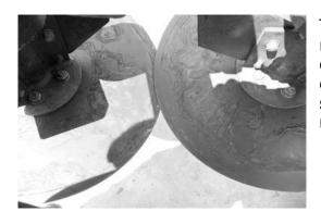
This shows overlap: generally, no less than 20mm and no more than 30mm. As discs wear, take note of which disc is wearing faster. This will be a guide as to which disc to adjust. e.g. Do not just adjust from the bump stop bolt, as you will end up with your cutting point misaligned to the required row spacing.
